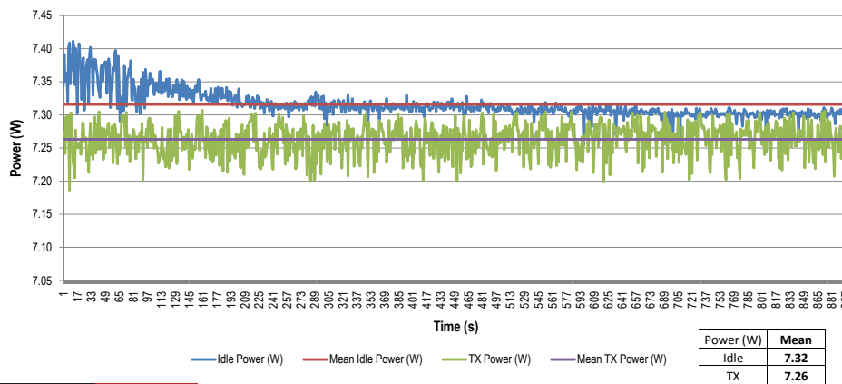
Linksys AG041 Idle & Transmit Power Levels
