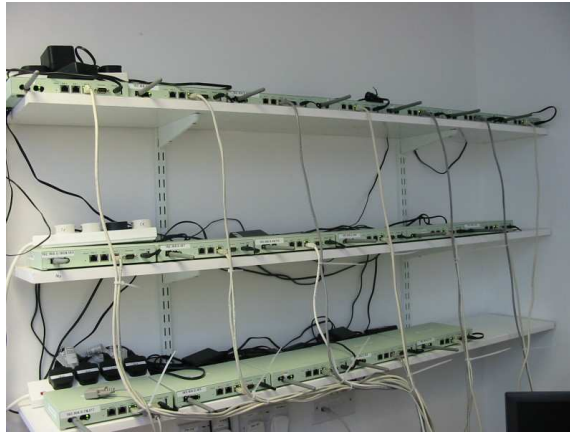
Figure: PC as AP, 1 PC and 9 PC-based Soekris Engineering net4801 as clients. All with Atheros AR5215 802.11b/g PCI cards. Modified MADWiFi wireless driver for fixed 11 Mbps transmissions and specified queue-size.
