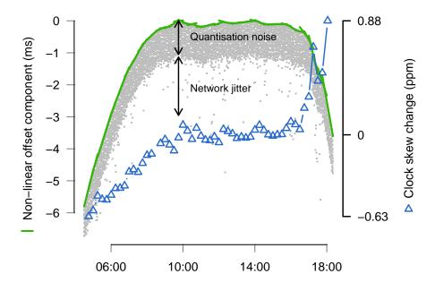
Many samples, over a long time, are needed to eliminate this noise
