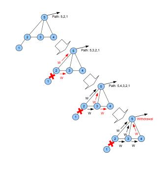
Fig. 1. BGP path hunting problem: The lost reachability of router 1 takes 3 update message before it is properly registered by router 5 (image borrowed from [2])
