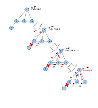
Fig. 1. BGP path hunting problem: The lost reachability of router 1 takes 3 update message before it is properly registered by router 5 (image borrowed from [2])
