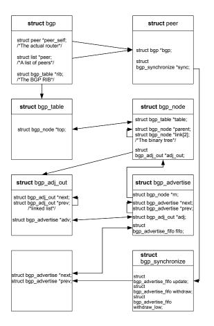
Fig. 2. A simplified diagram of struct interdependencies in bgpd
