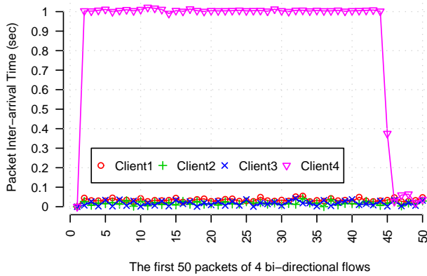
Fig. 32. Live Capture: HL2DM packet inter-arrival time
